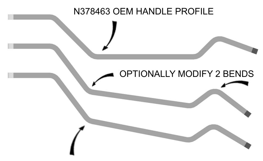
OPEN THIS ANGLE FOR USE ON CPIK76830 ANTI PLUG DOOR TO APPLY INCREASED PRESSURE TO CLOSE DOOR
